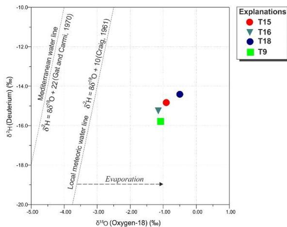
Figure 8: Isotope evaluation of the Tuzla geothermal waters
