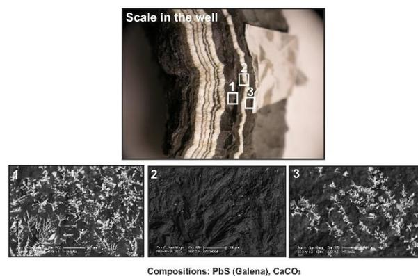
Figure 10: SEM analysis of the scale sample
