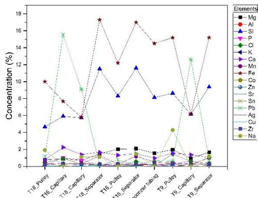
Figure 11: Elemental compositions of the scale sample
