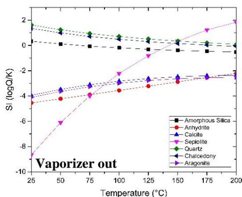
**Figure 12: Mineral saturation-temperature diagrams for the downholes and surface equipment system in the TGF**
